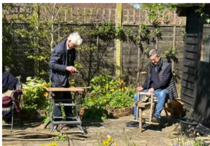
Green woodworking – using a shave horse and draw knife
